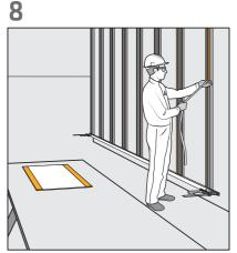
Remove the protective foil on the SikaTack® Panel Fixing Tape.
