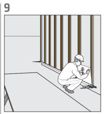
Place the cladding panel in the required position first, without the panel touching the fixing tape. After press it firmly until it touches the SikaTack® Panel fixing tape.
