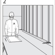
The surface to be bonded must be clean, dry and free from grease. Abrading with an abrasive pad (grain 80) on the panel and the substructure when recommended for the specific system.
