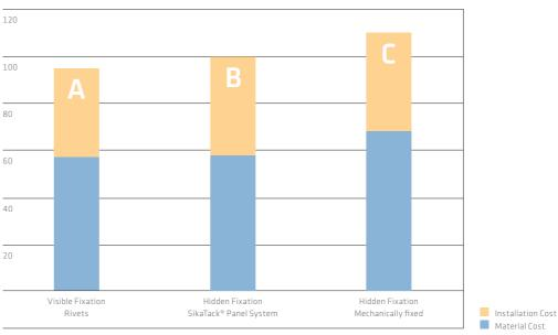
**Column A**: Visible fixation with rivets for an aluminium composite panel construction: total project cost separated into material – and installation cost .
