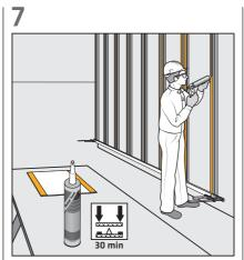
Apply SikaTack® Panel Adhesive in a triangular bead by using the triangular nozzle supplied (width 8 mm, height 10 mm) with at least 5 mm gap to the fixing tape and to the side of the batten.
