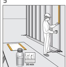
Shake SikaTack® Panel Primer thoroughly (the movement of the steel balls in the container must be clearly audible). Apply one thin coat of SikaTack® Panel Primer uniformly over the whole surface with a felt pad.
