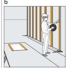
Apply SikaTack® Panel Fixing Tape over the whole length of the vertical sections and parallel to the edges.
