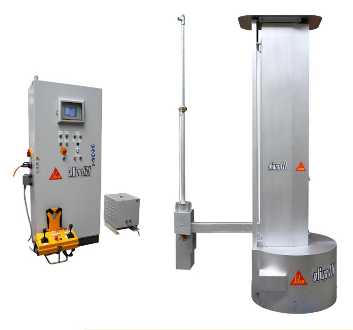
for hot or cold refractory repair for snorkels in vacuum plants automatically spraying inside more economical
